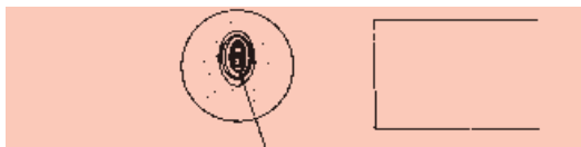
h) Note fatigue lines originate from the internal point, not outer diameter. Very rare failure type due to steel defect. 100% warranty accepted.
